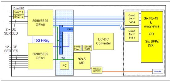
Figure 4-4 Nortel Networks L2/3 GbESM block diagram
